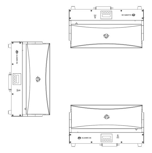
The Allegro Z6 is fully operational in three different mounting positions, hanging upside-down from a ceiling or trussing, sideways on trussing, or set on a flat level surface. Be sure this fixture is kept at least 12m (40ft) away from any flammable materials (decoration etc.). Always use and install the supplied safety cable as a safety measure to prevent accidental damage and/or injury in the event the clamp fails (see next page). Never use the carrying handles for secondary attachment.
