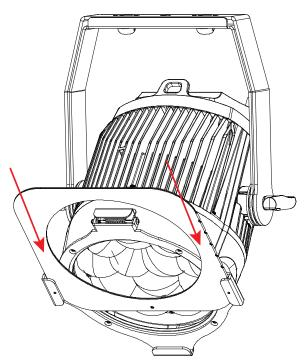
3. Slide the gel frame into gel frame holder's slot.
