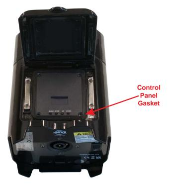
4. Reassemble the device by re-connecting the wire connector, then placing the display screen panel back in place. Please make sure that the gasket is fully seated around the edge of the panel. Replace the panel screws, and torque to **3.6 lb-in (4.2 kg-cm).**
