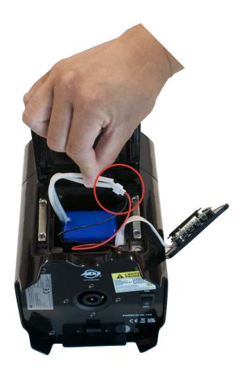
3. With the display screen panel removed, the blue colored battery should be plainly visible. Locate the two white wires that run from the battery and link to a red wire and a black wire via a small white connector. Disconnect the connector, then remove the battery and replace with a new unit.
