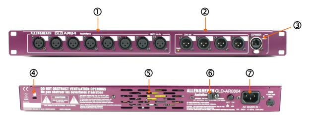
Input sockets 8 balanced XLR inputs for microphone and line level sources. The preamps are built into the AR84 rack and their Gain, Pad and 48V phantom power is remote controlled from the GLD console via the EXPANDER link. The output of the analogue preamps are converted to digital format and transported via a Cat5 cable to be processed and mixed at the GLD-80 mixer.
