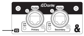
(i) The I/O Port panel is also used to access DIP switch 6 for network reset of the unit to default settings. Reset occurs with switch 6 in the On position at power up. After 10 seconds, turn off the unit and move the switch back to the Off position. Do not alter the position of the other DIP switches.
