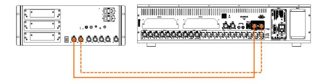
Switch on the Surface. The gigaACE Lnk/Err indicators flash at a steady rate when the link is established. The red error indicator lights if a communication error is detected. Check that the cables are correctly plugged in and are not faulty.
