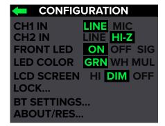
To change a setting, just rotate the speaker control knob until the configuration you desire to change is illuminated, then push to select it.
