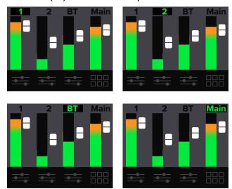
In order to change the level, push the speaker control knob when the desired channel is illuminated. In the example below, notice how the channel 2 fader has been moved to the -14 dB mark. Once the level you desire has been dialed in, press the speaker control knob again to return to the mixer screen.
