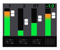
The top row selections change the levels of input channels 1, 2 and BT and the Main output. Notice below how each parameter illuminates as the speaker control knob is rotated to the right from channel 1 to 2, Bluetooth (BT) and the Main output last.
