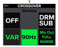
Also available is a mix out mode. The mix out mode allows you to select if the signal passes all frequencies (Full Range) or only the low frequencies (Low Pass) out of the mix out jack, acting as a fixed or variable system crossover for full range systems where the audio is routed first through the V-Class, and then to the sub. Push the speaker control knob in and release to switch between the two mix out mode selections. Release when the one you desire is illuminated, then leave it be.
