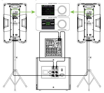
If you desire a little more boom, add a DRM18S subwoofer to the mix. Here, the L/R outputs of a ProFX10v3 mixer are connected directly to the channel 1 and 2 inputs of the DRM18S subwoofer. Then the High-Pass Outs of the subwoofer are connected to the channel 1 inputs of a pair of SRM212 | V-Class loudspeakers. The gain knob on both should be set to Line. Here you will want to set the Speaker Mode to either Live or Club and the Subwoofer HPF to DRM Sub (or Var if using a different subwoofer).
