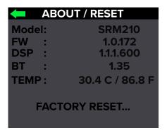
The first two items display the loudspeaker's firmware and DSP versions and the third is the temperature of the loudspeaker. None of these are editable, but they could come in handy if you need to talk to someone in Technical Support.
