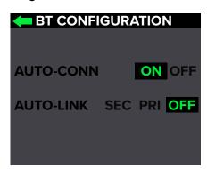
**Auto Conn** – Allows a previously paired device to auto reconnect if both the device and speaker are powered on and in range. When illuminated, push the speaker control knob to select between on or off.
