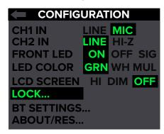
**Locking** – Push the speaker control knob to enter lock mode. From here, rotate the speaker control knob until the first number you desire is illuminated and press to select. Follow the same procedure for the next three numbers.
