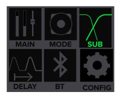
• Var – Choose this if a non-Mackie DRM18S subwoofer is connected to the system. Here you can select the subwoofer's HPF, ranging from 40 Hz – 160 Hz.
