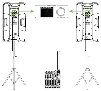
In this example, a ProFX10v3 mixer is connected directly to two SRM212 | V-Class loudspeakers. It is the perfect setup for a small club or... a fun karaoke house party! Simply connect the L/R outputs of the ProFX10v3 mixer to the channel 1 input of each SRM212 | V-Class loudspeaker. The gain knob on both should be set to Line. Don't forget to set the Speaker Mode on both loudspeakers to Live... or Club if you want a little more low-end thump!
