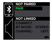
(2) The text "NOT PAIRED" will change to "DISCOVERABLE" and "PAIR" will change to "CANCEL". From here, you can either (A) turn the device and device's bluetooth on to pair, or (B) push the speaker control knob to cancel the action.
