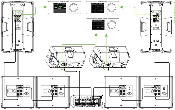
Here's how to set up a large club system. In this example, the L/R outputs of a DL16S mixer are connected directly to the channel 1 inputs of a pair of DRM18S subwoofers. The Direct Out of each subwoofer is then connected to the inputs of an additional pair of DRM18S subwoofers.
