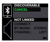
(3) The text "DISCOVERABLE" will change to "PAIRED" and "CANCEL" will change to "DISCONNECT". From here, you can either (A) use the device and SRM Connect app to control the loudspeakers, or (B) push the speaker control knob to disconnect.
